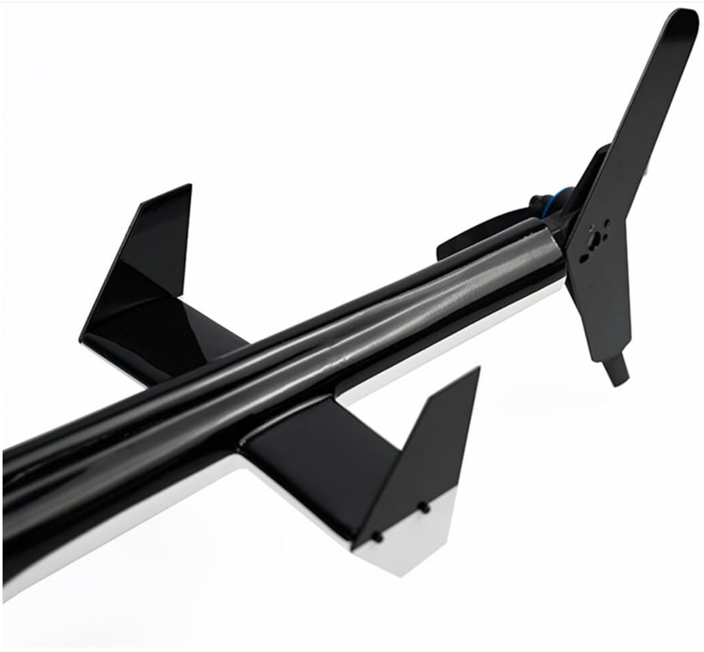
Figure 7.1: Detailed view of the tail rotor, an important component for flight stability and requiring regular inspection.
