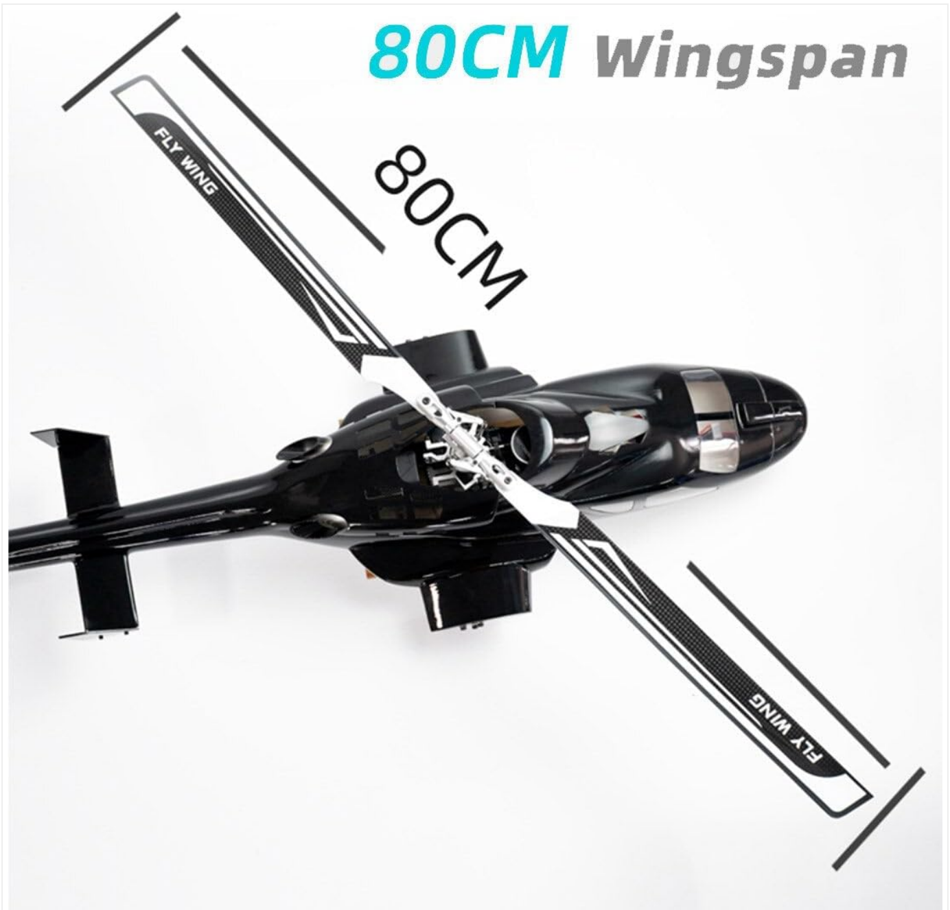
Figure 4.1: The FW450L Airwolf helicopter highlighting its 80cm wingspan (main rotor diameter).
