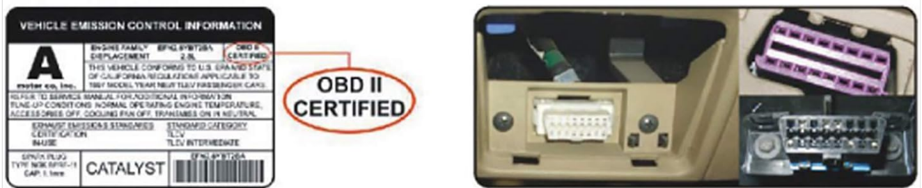
Figure 5: Example of an OBDII certified sticker and the typical location of the 16-pin diagnostic link under the dashboard.
