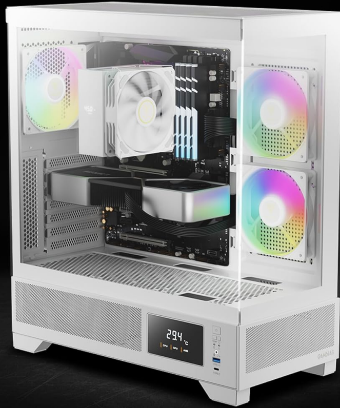
Figure 4.7: View of the pre-installed ARGB PWM fans within the case.
