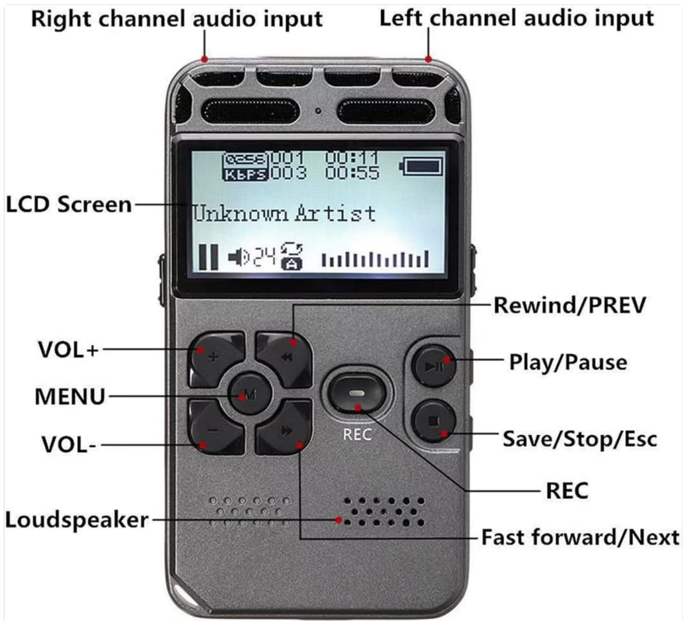
Figure 2: Labeled diagram of the SK-502 Digital Voice Recorder controls and ports.
