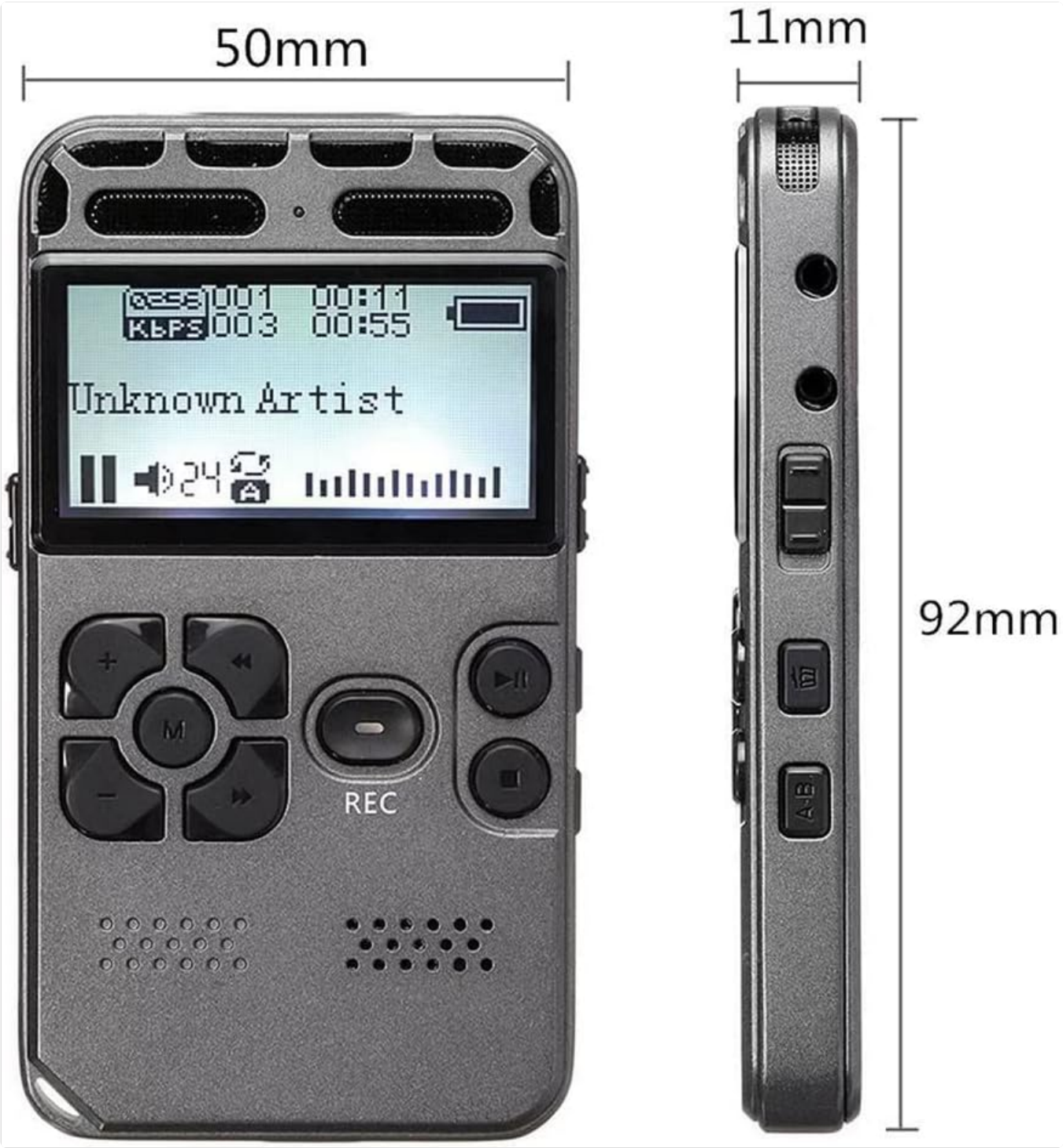
Figure 4: Detailed dimensions of the SK-502 Digital Voice Recorder.
