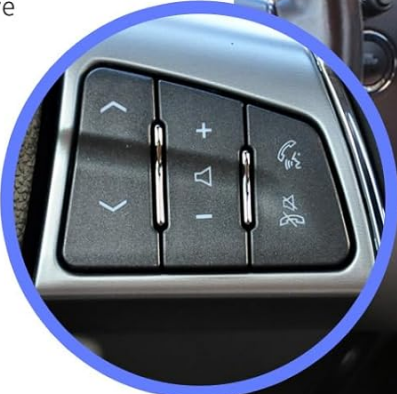
Figure 8: Utilize your vehicle's existing steering wheel controls for convenient and safe operation of the head unit.
