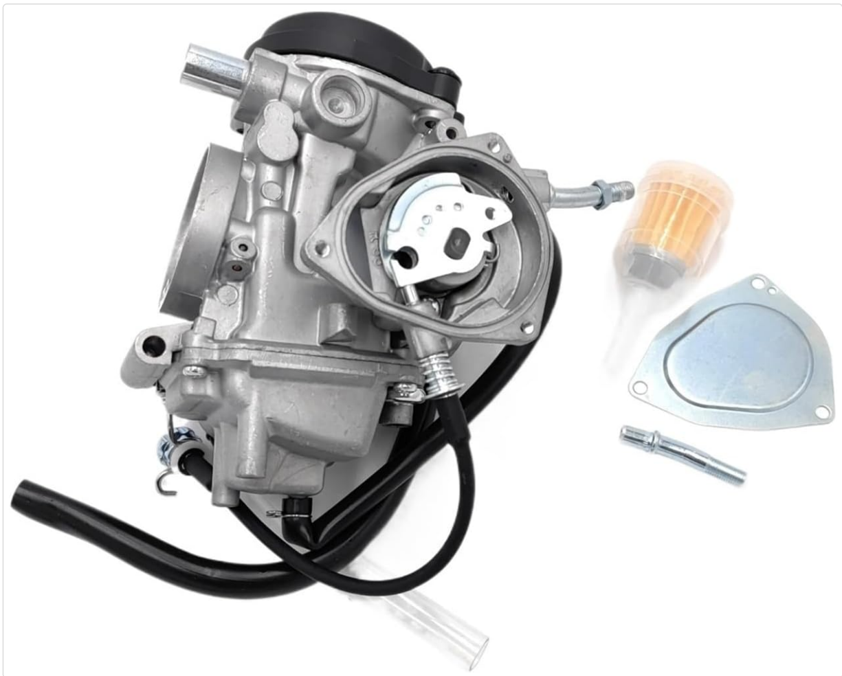
Figure 4: View of the carburetor's throttle linkage and choke mechanism, essential for engine control.
