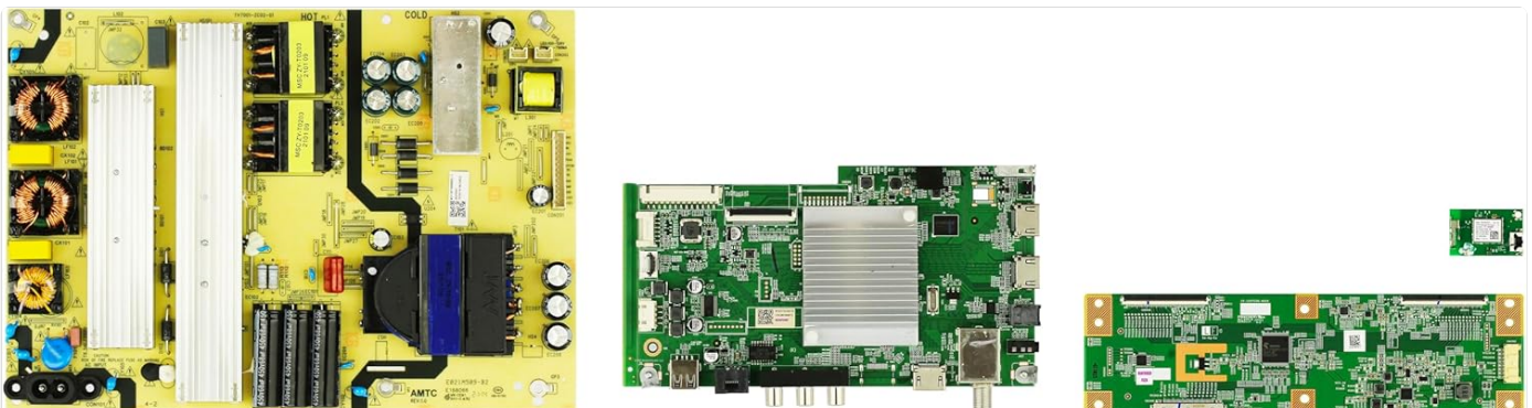
Figure 1: Components of the ONN 100012588 TV Repair Parts Kit. This image displays the power supply board (left), main board (center),
