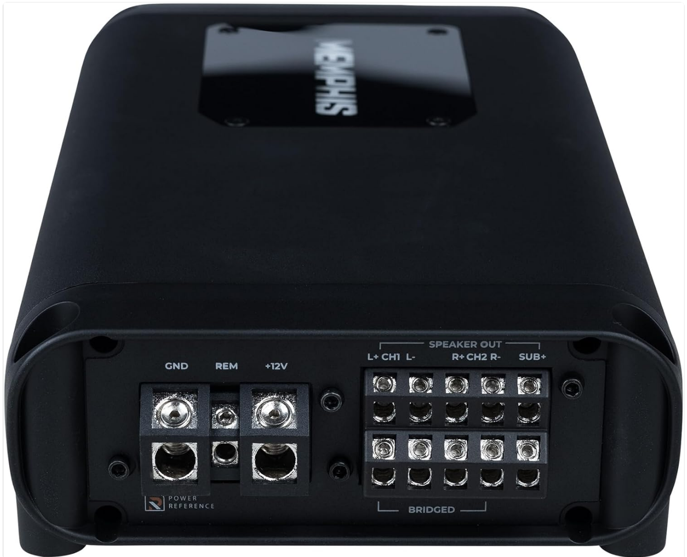
Figure 3: Close-up view of the power and speaker output terminals, including bridged connection options.
