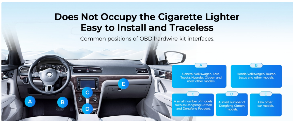
Image: Common OBD port locations in various car models.
