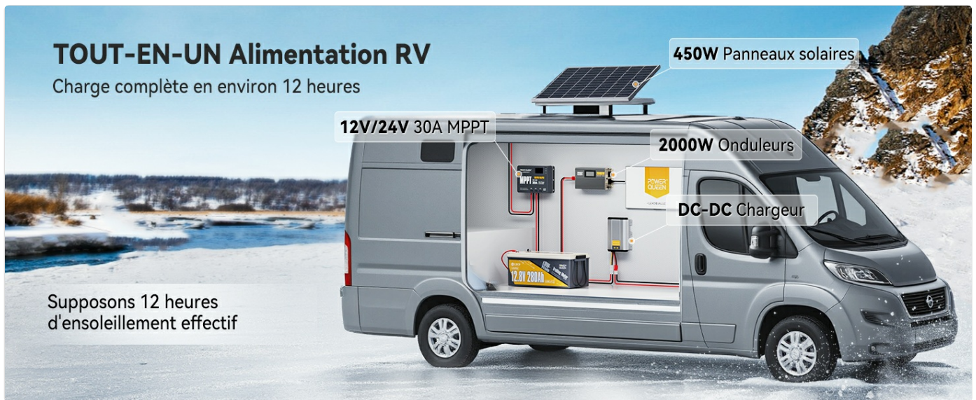
Image 5.1: Example of an RV power system utilizing solar panels for charging.
