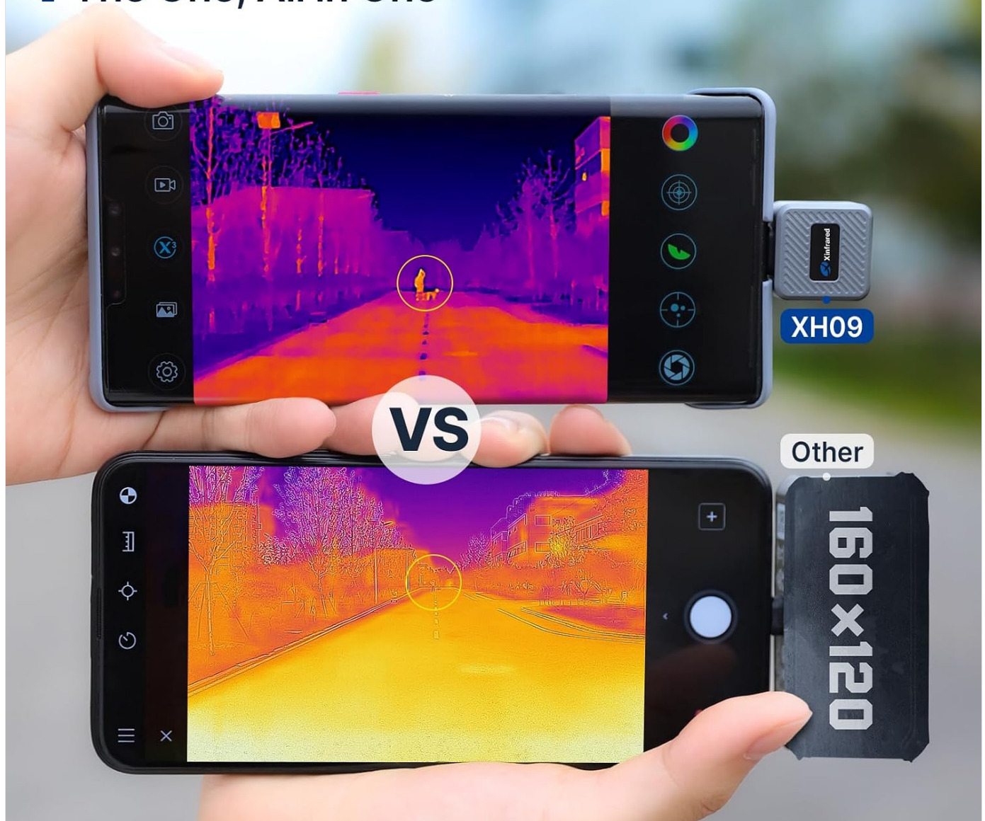
Figure 3.3: Visual comparison demonstrating the XH09's 870m detection capability. The top image shows a clear thermal outline of a person at a distance using the XH09, while the bottom image from another device shows less detail.
