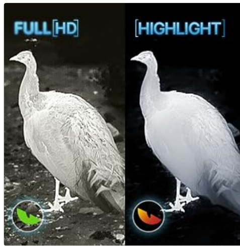
Figure 3.12: A side-by-side comparison of Full HD and Highlight thermal imaging modes. The left image shows a detailed thermal view of a peacock in Full HD, while the right image in Highlight mode emphasizes the thermal signature for easier detection.
