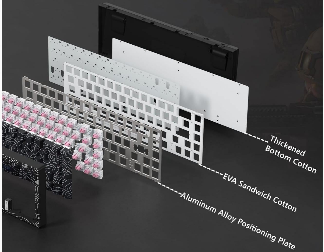
Figure 8: Internal Structure of the Womier M68 HE Keyboard.
