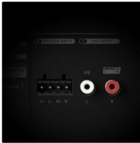
Figure 5: Close-up of the input panel on the KEF Kube 15 MIE. This image clearly shows the Speaker Input terminals, LFE (L) input, and Line Input (L/R) with the SmartConnect feature highlighted.
