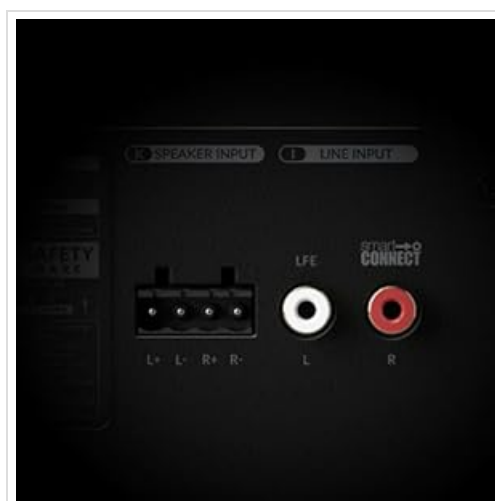
Detailed view of the SmartConnect and Line Input (LFE, L, R) ports on the subwoofer's rear panel.
