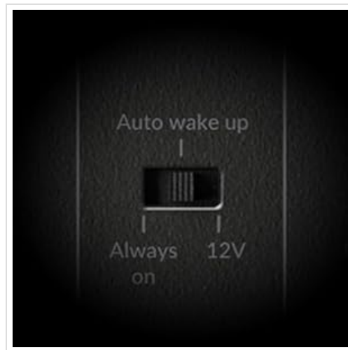
Detail of the Auto Wake Up switch, offering "Always on", "Auto wake up", and "12V" options.
