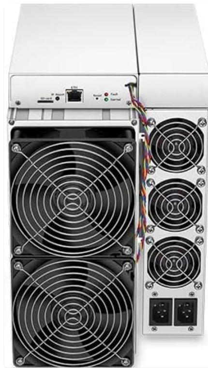
Figure 3: Rear panel of the Antminer S19, highlighting power input ports and the RJ45 Ethernet port.
