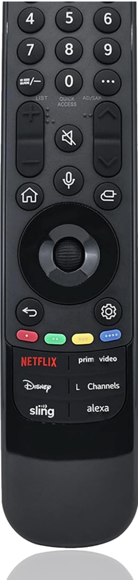
Image 2.1: Front and side view of the MR23GA Magic Remote Control, showcasing its ergonomic design and button layout.
