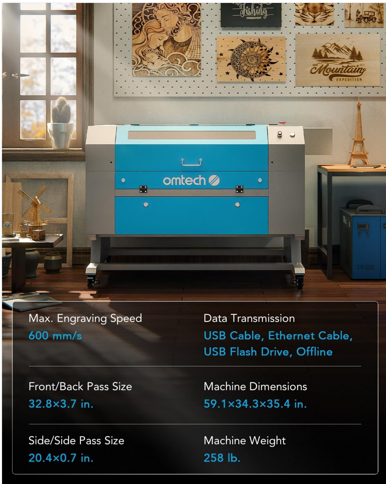
Image 8.1: Overview of the OMTech 90W CO2 Laser Engraver's key specifications and features.
