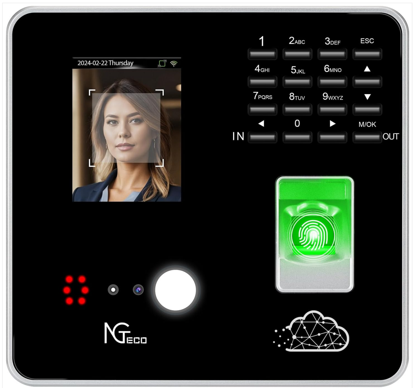
Figure 1: Front view of the NGTeco TC1 Cloud Time Clock, showing the facial recognition camera, fingerprint scanner, keypad, and display.
