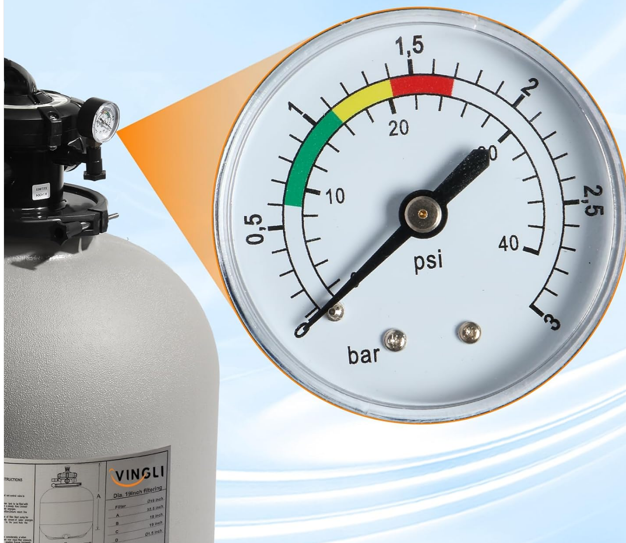
Figure 6: The pressure gauge indicates the filter's internal pressure. A higher reading (e.g., above 1.5 bar) suggests backwashing is required.
