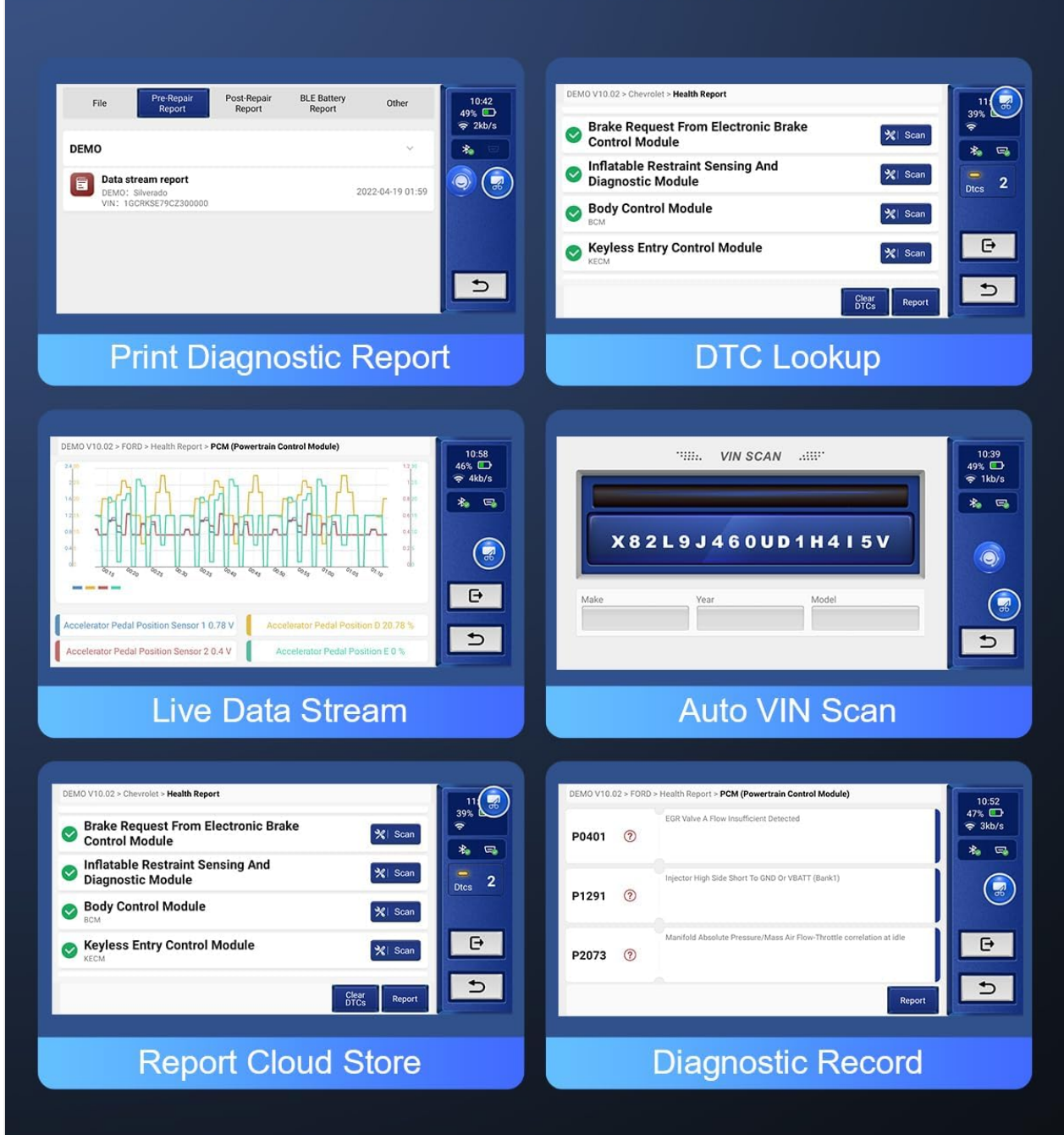
Figure 4.3: Intelligent Diagnostic Report. This image shows examples of the diagnostic report interface, including options to print reports, look up DTCs, view live data streams, perform auto VIN scans, and manage diagnostic records.
