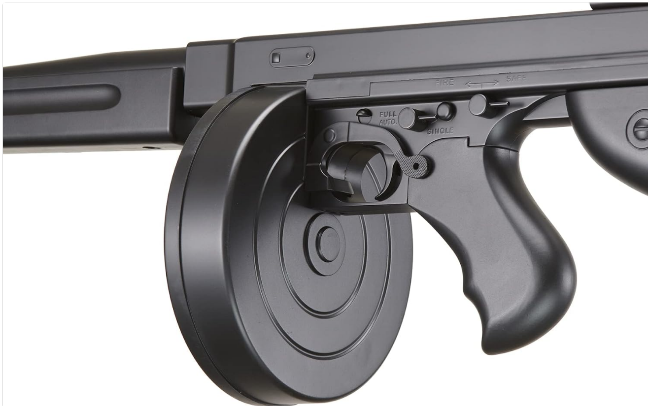
Figure 5: Detail of the safety and fire selector, showing "FIRE", "SAFE", "FULL AUTO", and "SINGLE" settings.
