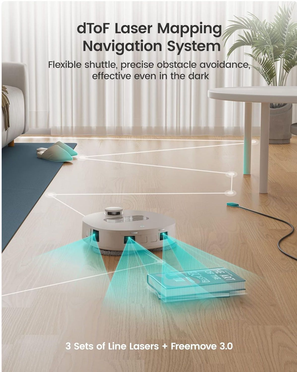
Image: The Lefant T1 robot mop navigating a room, illustrating its dToF laser mapping system with light beams detecting obstacles and mapping the environment.
