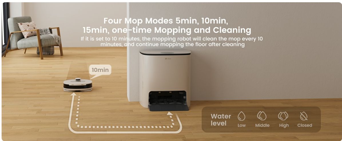
Image: The Lefant T1 robot mop returning to its base station, illustrating the "Four Mop Modes" (5min, 10min, 15min) for automatic mop cleaning frequency, along with water level settings (Low, Middle, High, Closed).
