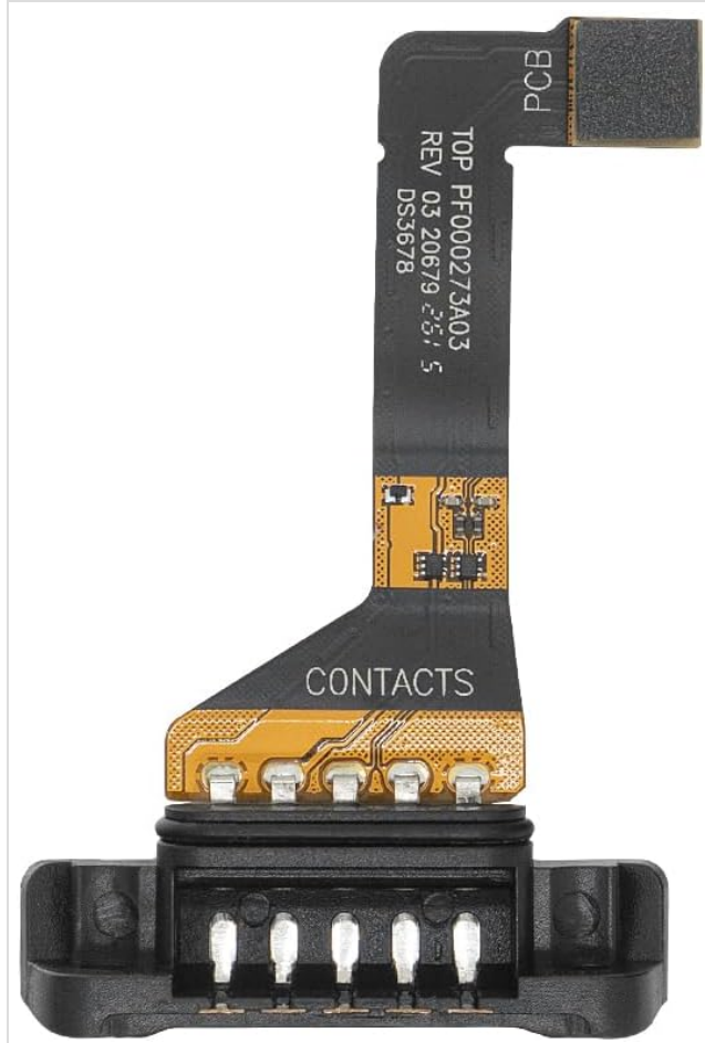
Figure 2.2: Rear view of the connector, displaying the printed circuit board (PCB) and internal contact points.
