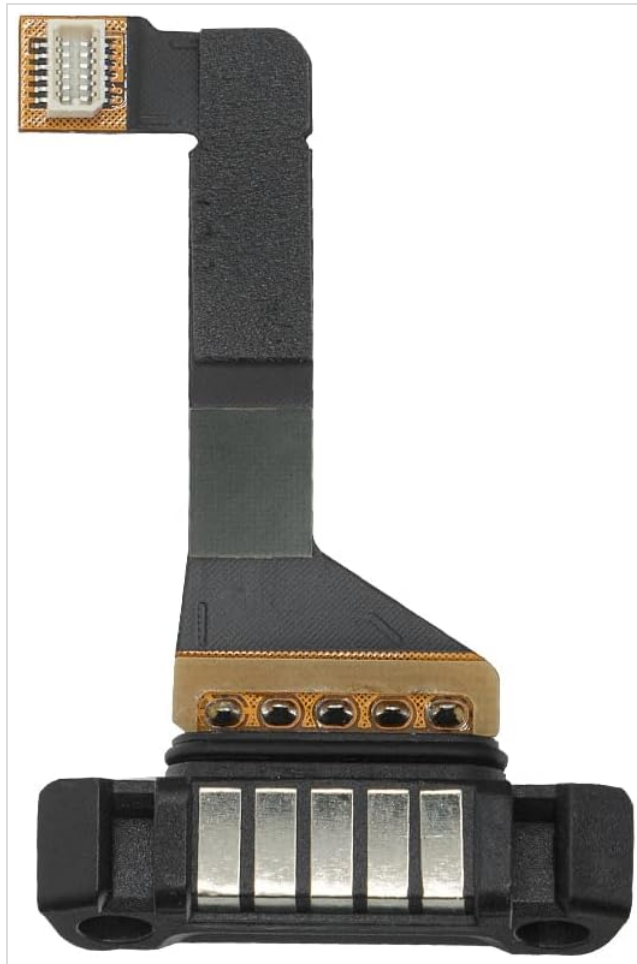
Figure 2.1: Front view of the 5-pin charging connector, highlighting the metallic contact pads.
