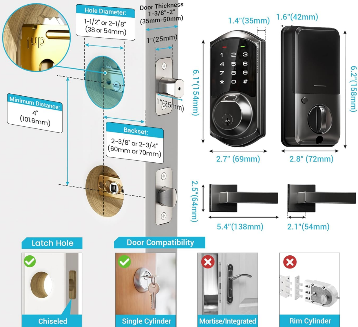
Figure 2: Door Size and Compatibility Requirements
