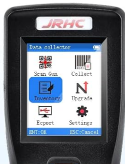
Image 5.1: The JRHC S-8103T scanner in operation, highlighting its ability to read various 1D and 2D barcode types, including QR codes and PDF417.
