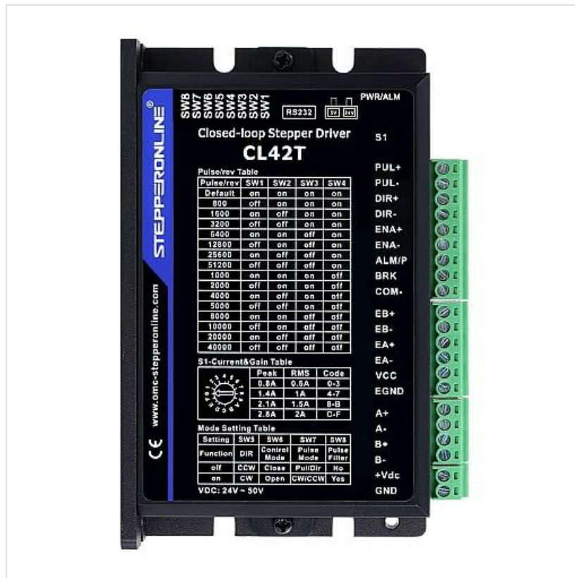
Figure 4: CL42T Closed Loop Stepper Driver. This image displays the driver unit, showing its various input/output terminals and DIP switches for configuration.
