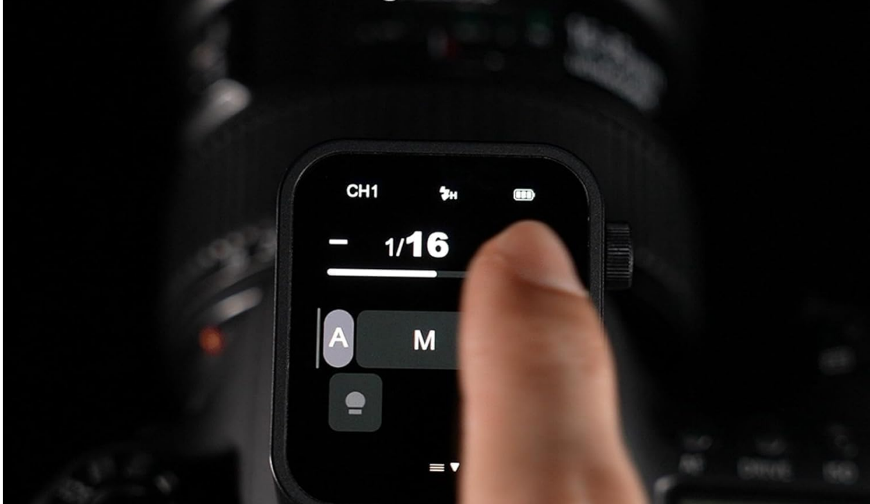
Image: The X3-C's screen showing the TCM function, allowing for quick conversion of TTL settings to manual power.
