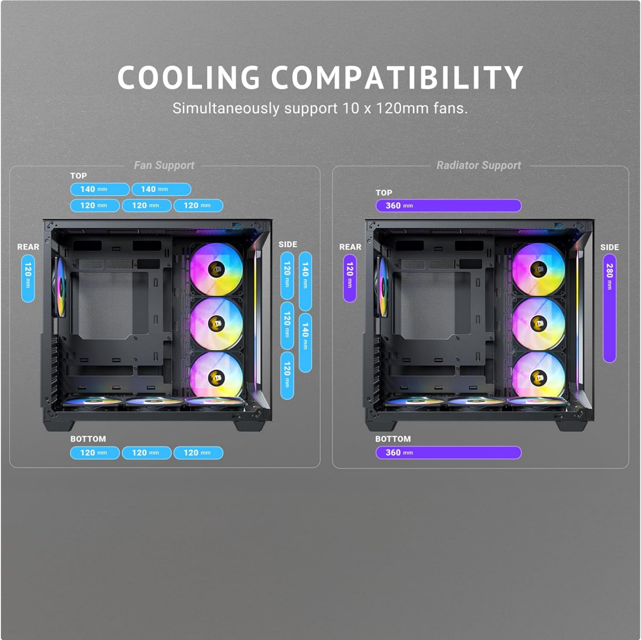
Image: Diagrams detailing the fan and radiator support locations and sizes within the Antec C5 ARGB case.
