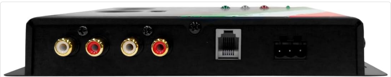
Figure 4.2: Rear panel connections. From left to right: RCA input jacks (red and white), RCA output jacks (red and white), remote bass level control port (RJ-11), and the power/remot turn-on connector.
