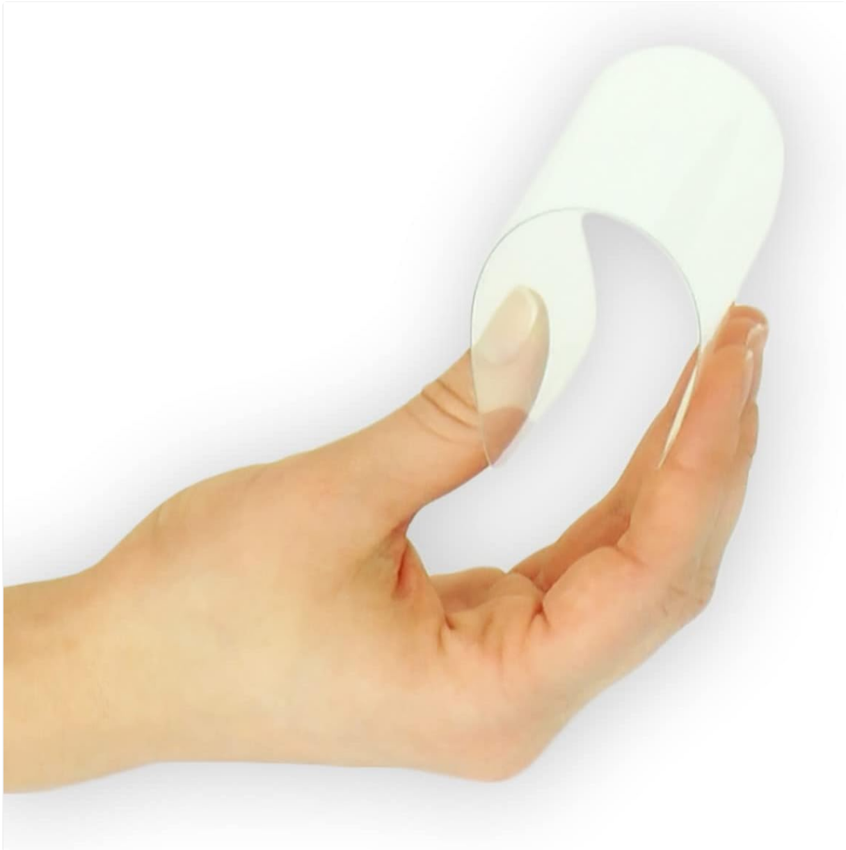
Figure 4: The flexible nature of the hybrid glass material.
