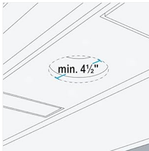
Image 2: Ensure a minimum 4.5-inch diameter hole is cut in the soffit.
