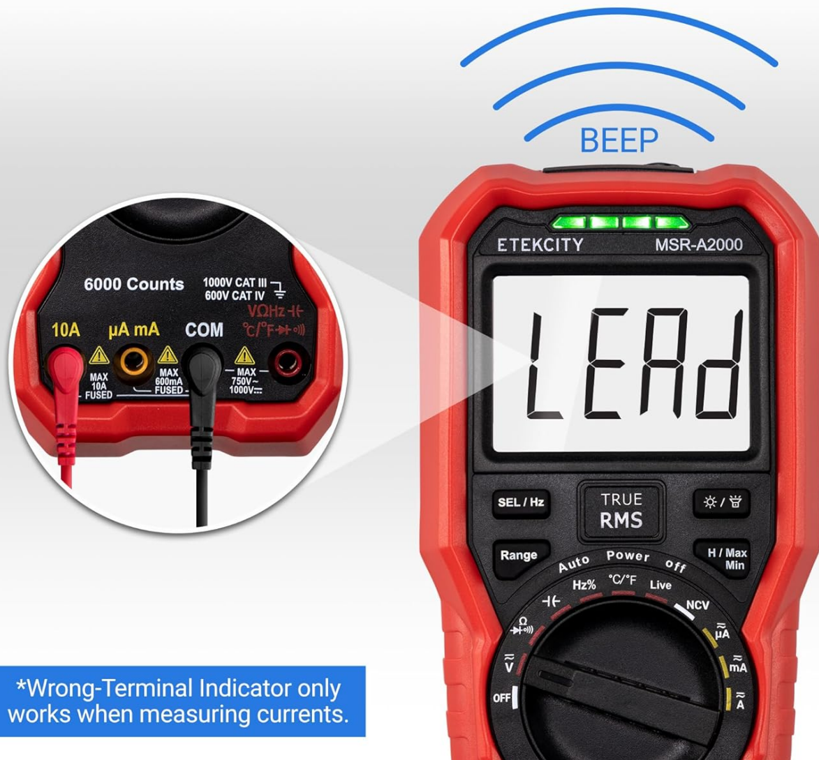
Figure 6: The Wrong-Terminal Indicator provides a safety alert.
