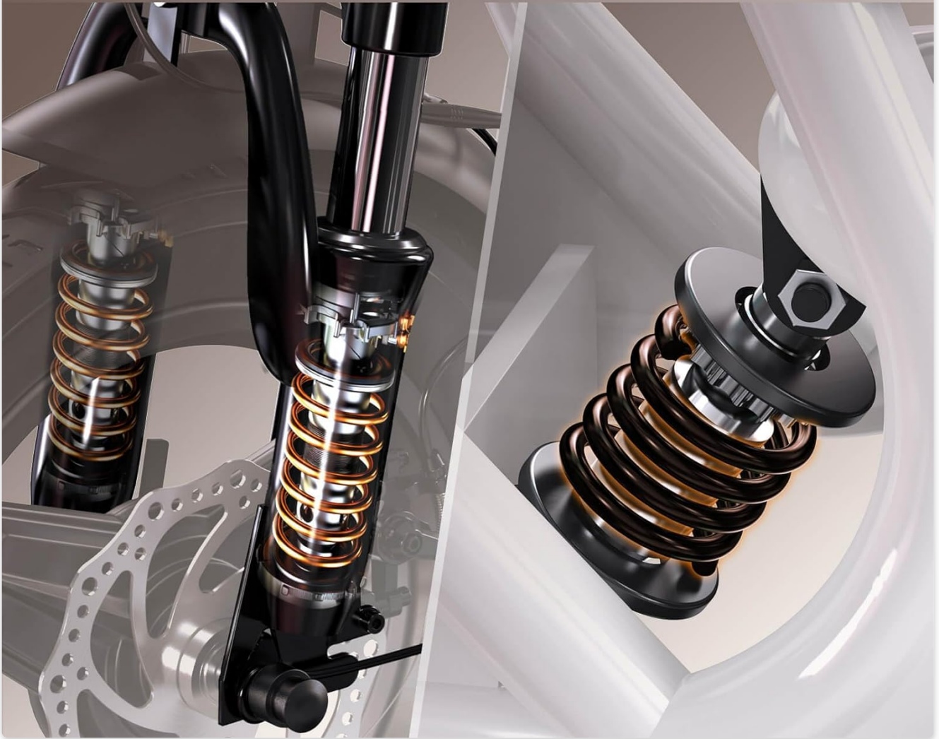
Image 7.2: The full suspension system ensures a comfortable ride by absorbing shocks.
