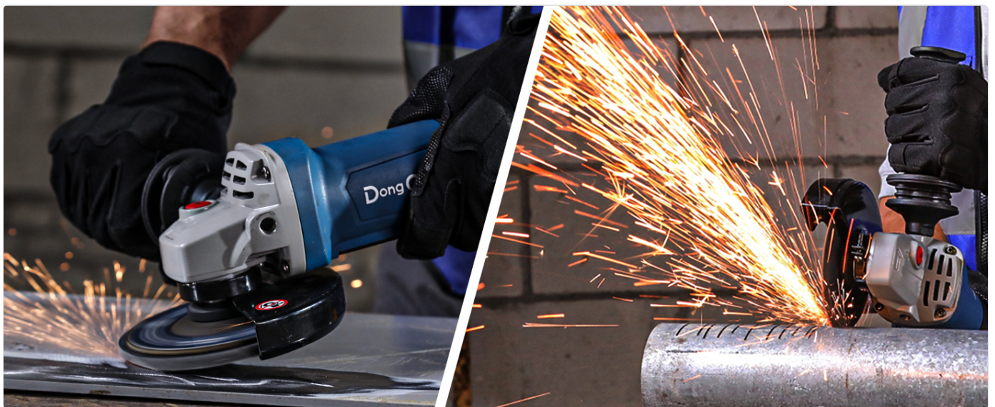
Figure 8: Angle grinder in action, demonstrating cutting with sparks.
