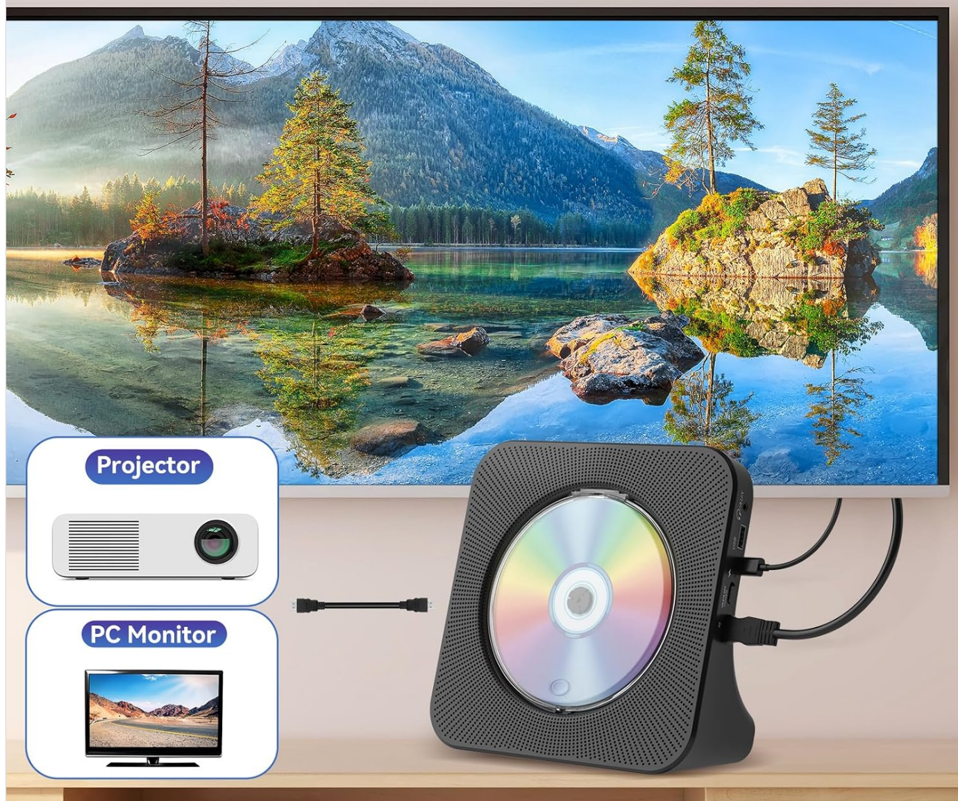
Image 3: Connecting the player to a TV, projector, or PC monitor using the HDMI cable.
