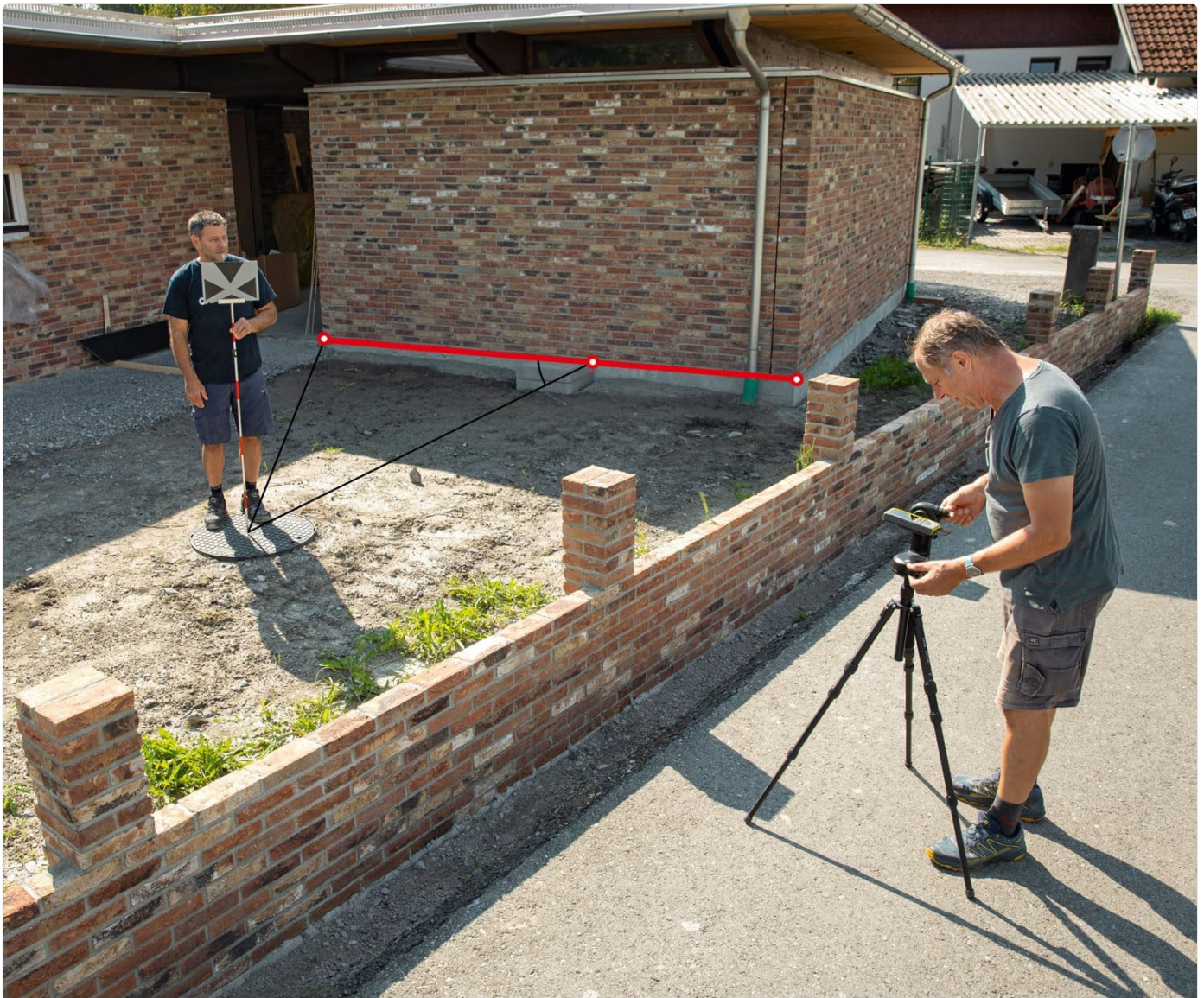
Figure 3: Example of the Leica DISTO X6 utilizing P2P technology to measure inaccessible areas, demonstrating its capability for remote and complex measurements.
