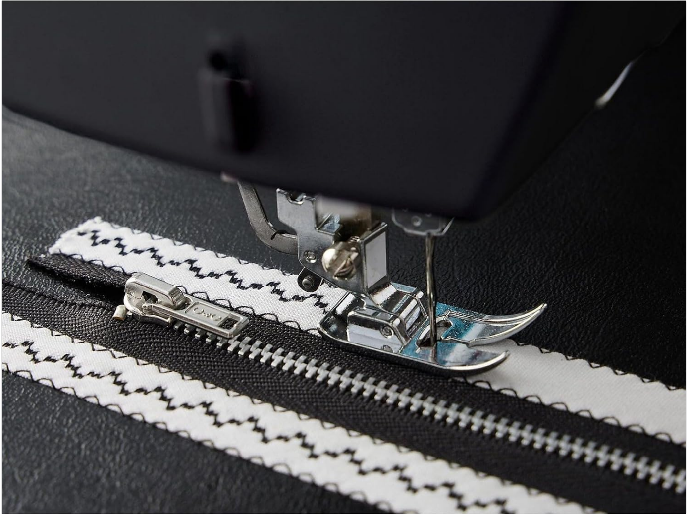
Figure 4.1: The machine in operation, demonstrating the use of a zipper foot for precise stitching alongside a zipper.
