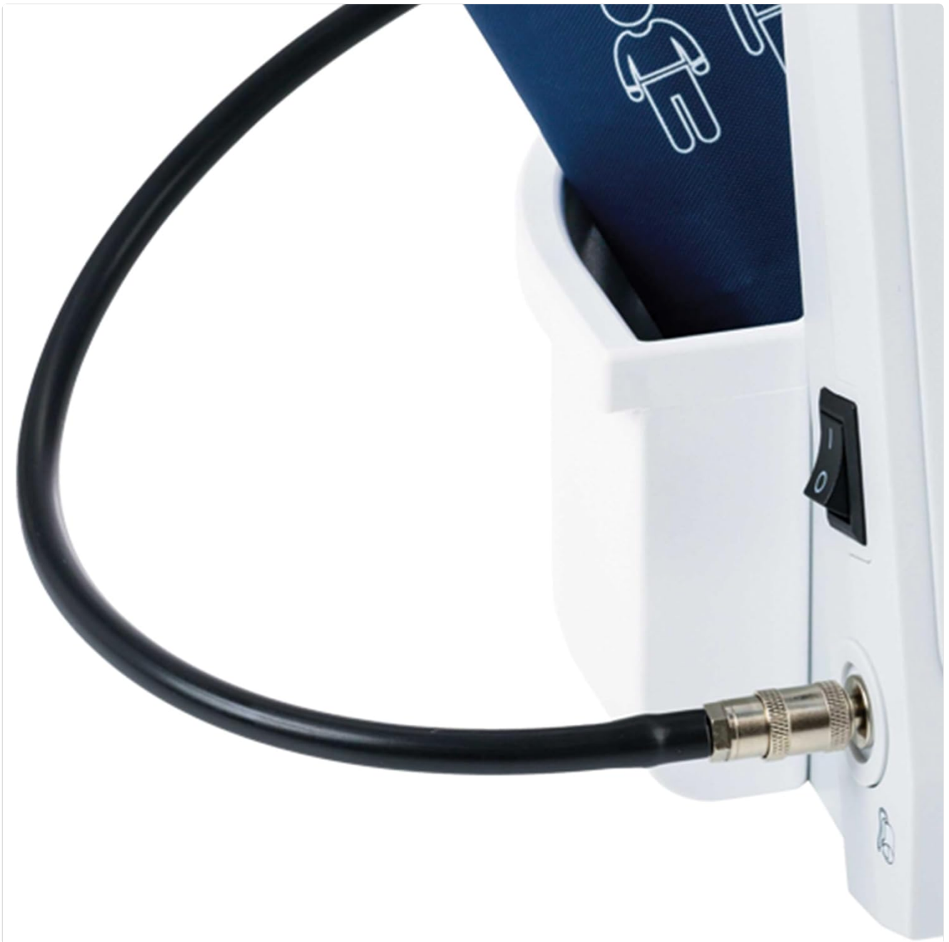
Figure 2: Detail of the cuff connection and power switch. This image shows the black air tube connected to the monitor's port, and the power switch positioned above it, indicating the device is ready for operation.
