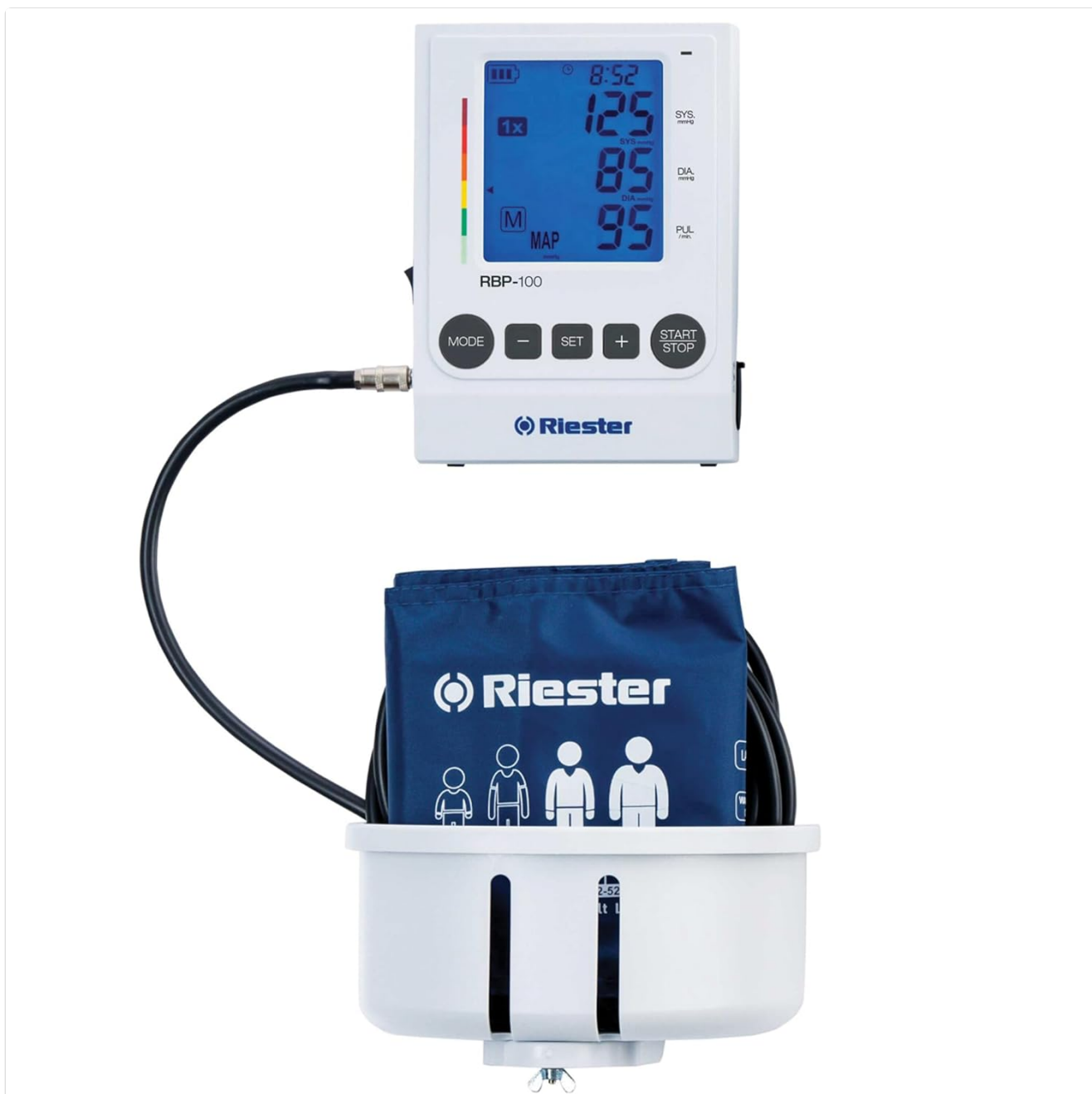
Figure 3: The RBP 100 monitor with its cuff stored in the integrated holder. This image provides a clear view of the monitor's display and control buttons, along with the connected cuff, illustrating its wall-mounted configuration.
