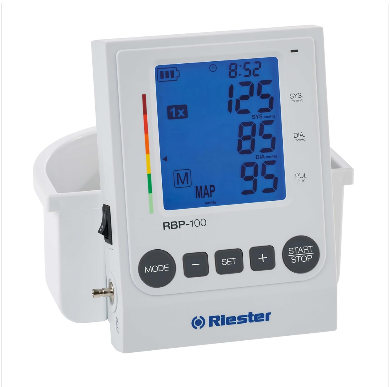
Figure 5: A detailed view of the RBP 100's digital display. The screen shows current time (8:52), battery level, and large numerical readings for systolic (125 mmHg), diastolic (85 mmHg), and MAP (95 mmHg) pressures, along with pulse rate. A color-coded WHO classification bar is visible on the left.
