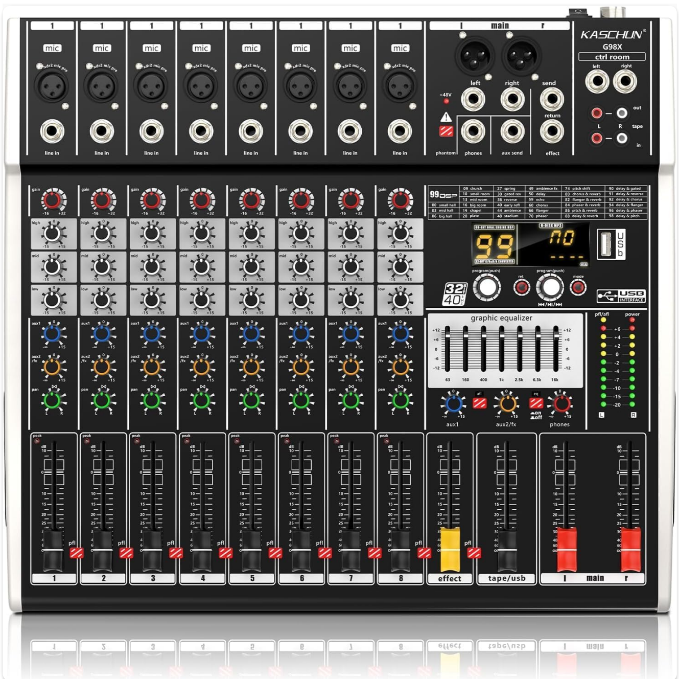
Figure 1: Kaschun G98X Professional 8-Channel Audio Mixer Overview
