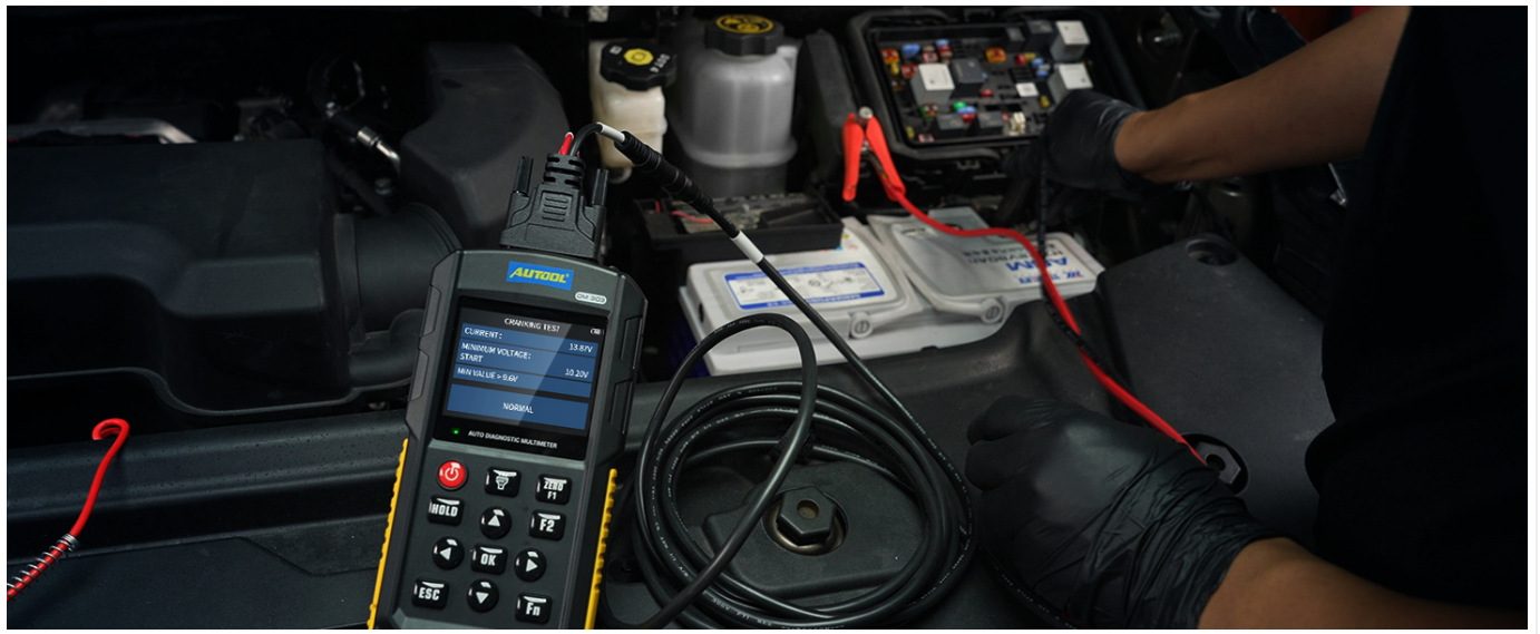
Figure 3.3: Cranking test in progress, showing the device connected to the car battery.
