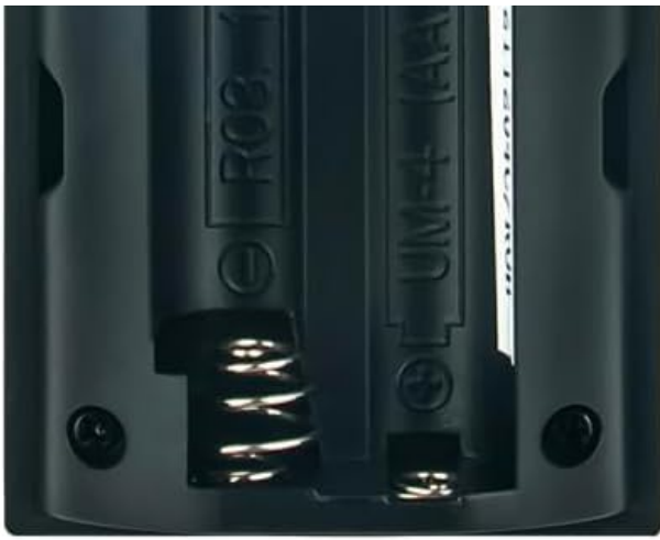
Figure 2: Rear view of the remote control with the battery compartment open, showing where to insert two AAA batteries.
