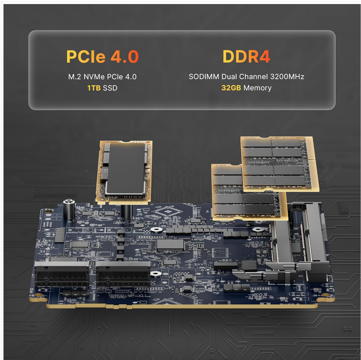
Figure 8: The motherboard with accessible slots for RAM and SSD upgrades.
