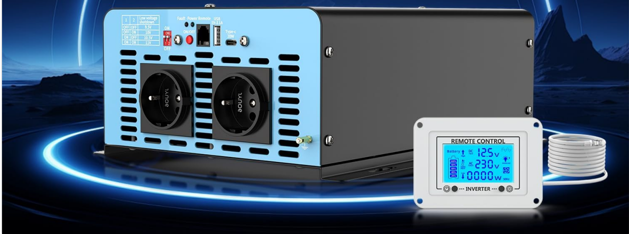
Figure 3.3: The remote control with its LCD screen. This display provides real-time information on battery status, DC input voltage, AC output voltage, current power consumption (in Watts), and indicators for overheat or overload conditions. Flashing icons on the LCD directly communicate any issues, aiding in troubleshooting and parameter adjustment.
