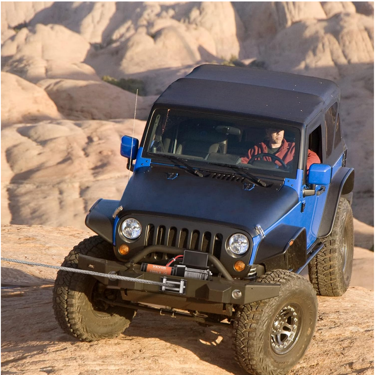
Figure 3.1: VEVOR 3000 lb Electric Winch. This image shows the complete winch unit with the steel cable spooled, the hook attached, and the fairlead mechanism.
