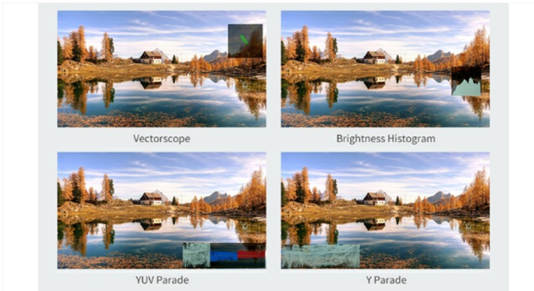
Image: A display of the FW568 PRO screen showing various monitoring tools including Vectorscope, Brightness Histogram, YUV Parade, and Y Parade, used for detailed video analysis.
