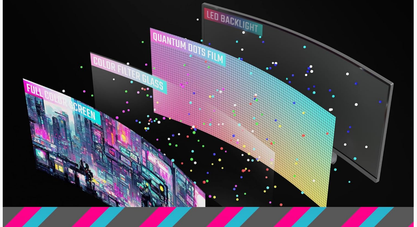
Figure 3.1: Diagram illustrating Quantum Dot display technology layers.
