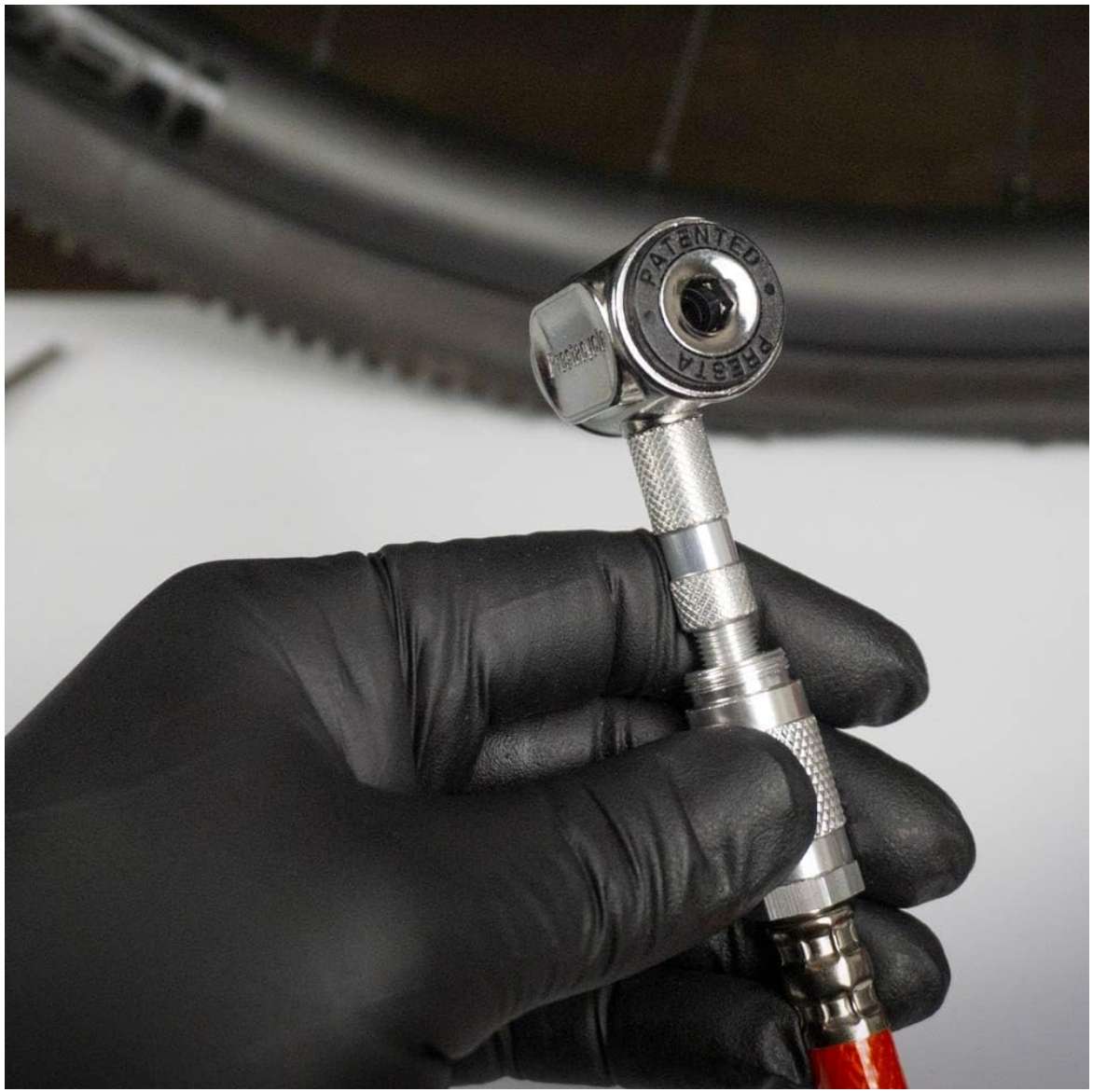
Image 3.1: Demonstrating the auto-lock connection of the Pro Presta Head to a Presta valve.
