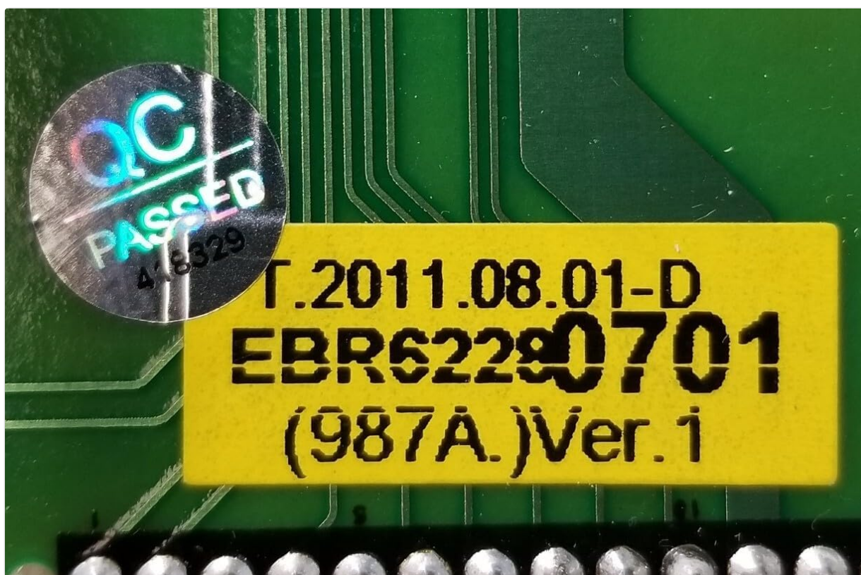
Figure 2: Close-up view of the part number label on the control board, showing 'EBR62280701'. Always confirm the part number on your existing board matches the replacement.
