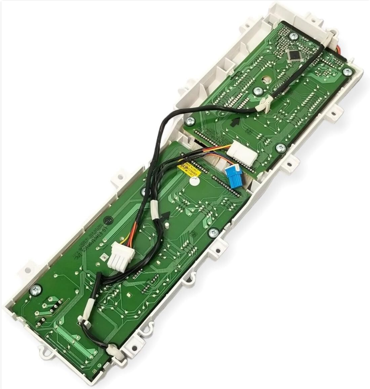
Figure 1: Generic Replacement Display Control Board EBR62280701 for Kenmore Washer. This image shows the full control board with its various electronic components and wiring harnesses.
