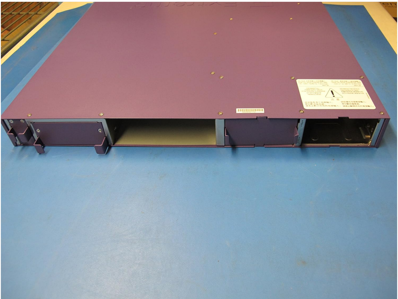
Image: Rear view of the Extreme Networks Summit X460-G2-48T-10GE4 switch, displaying two empty bays designed for hot-swappable power supply units.
