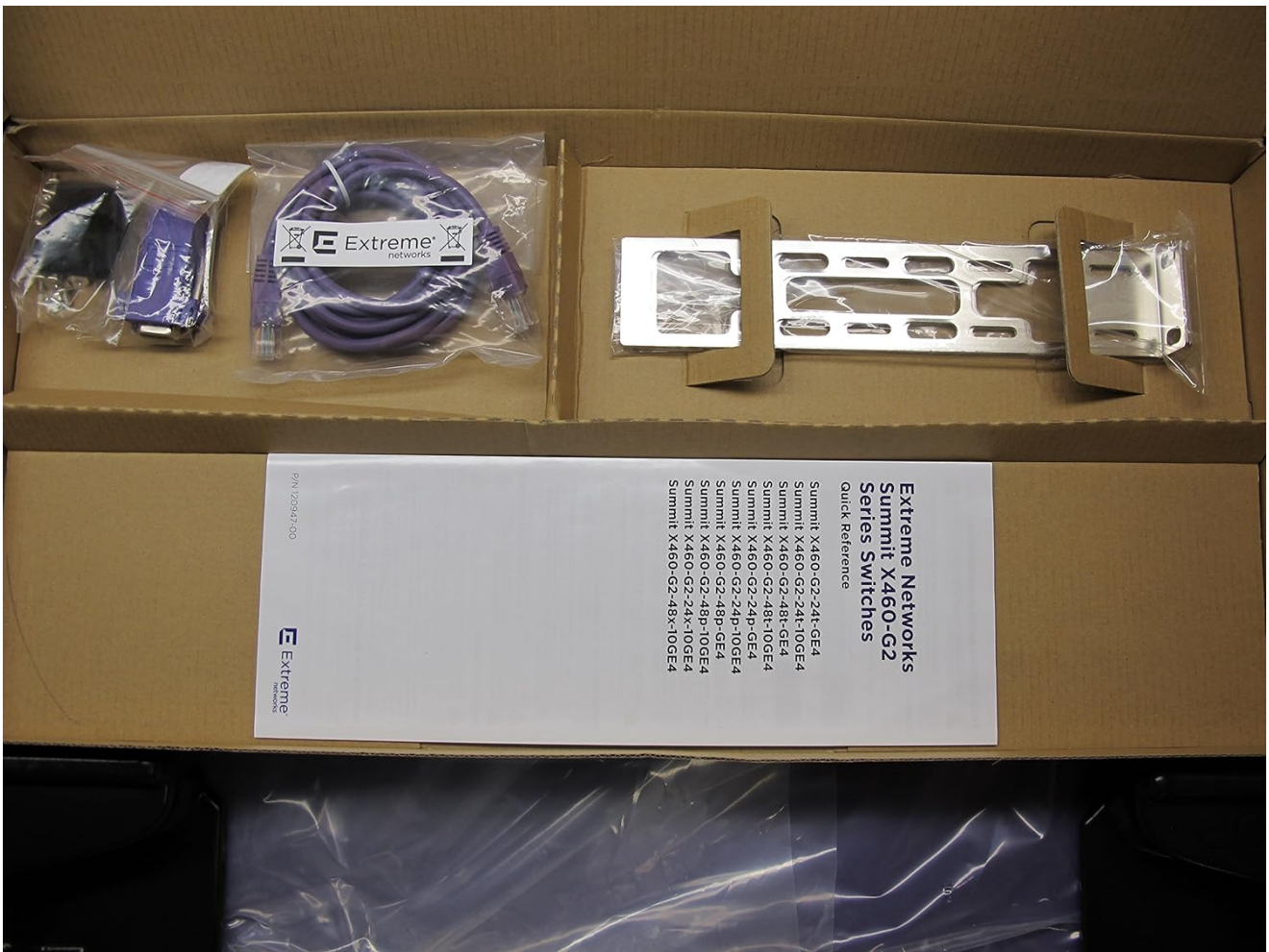
Image: Unboxed components of the switch, showing the main unit, a purple console cable, a power cable, rackmount brackets, and a Quick Reference Guide for Summit X460-G2 Series Switches.
