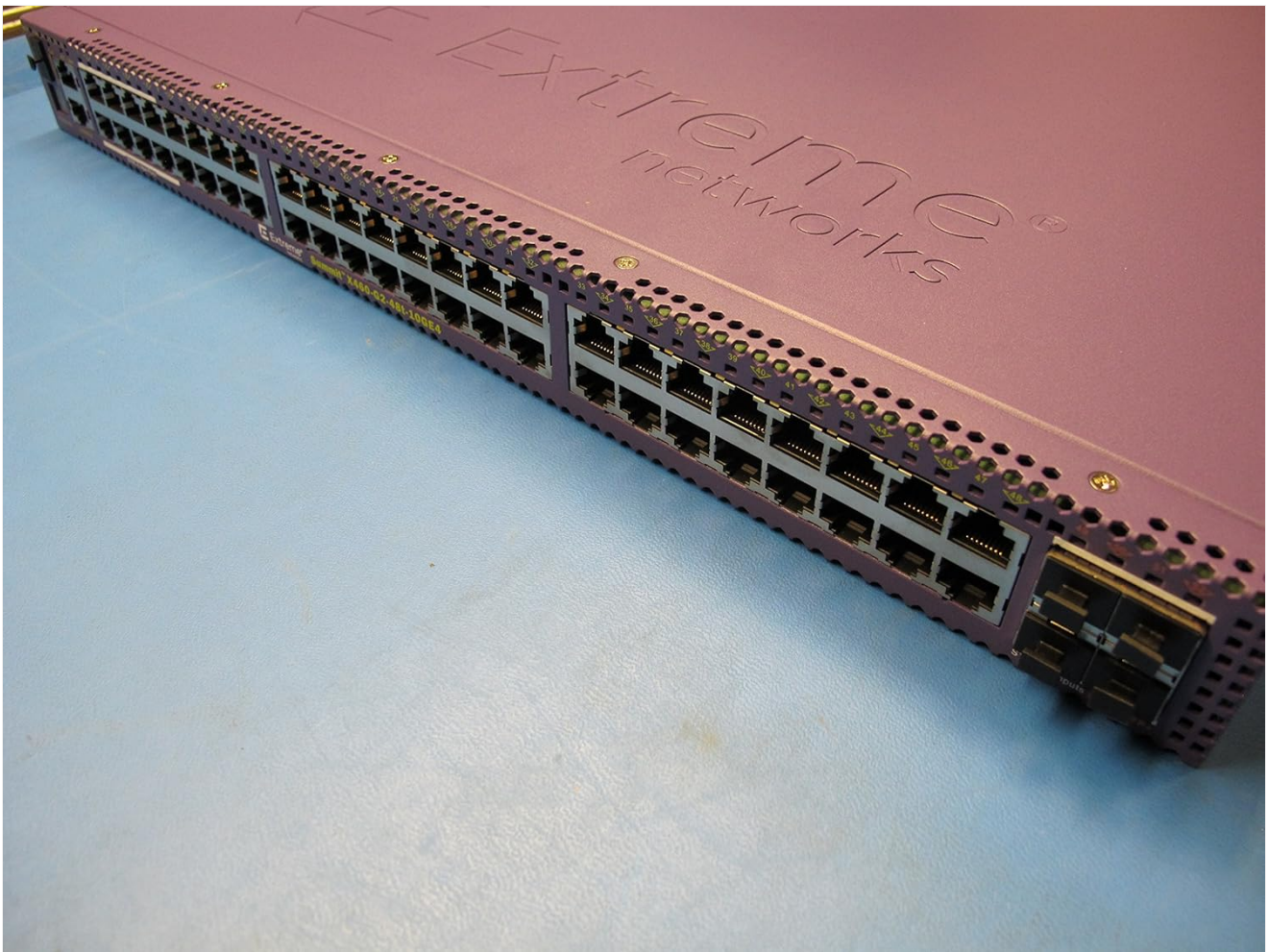
Image: Front perspective of the Extreme Networks Summit X460-G2-48T-10GE4 switch, highlighting the array of 48 copper Gigabit Ethernet ports and the four SFP+ transceiver slots on the right side.
