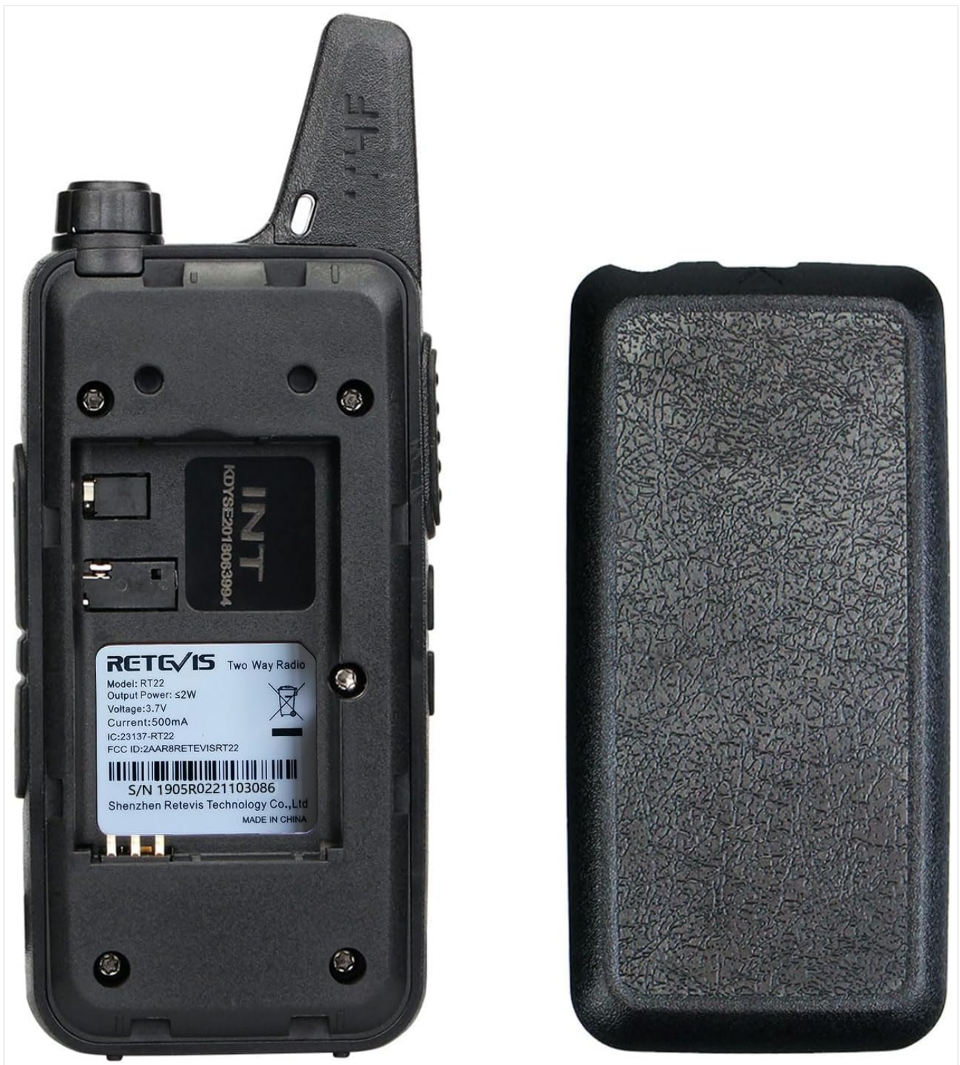
Image: View of the RT22 radio's battery compartment for installation.
